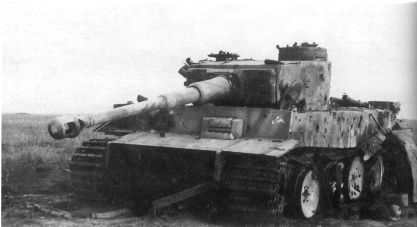
▼ Another shot of the same tank showing the Raging Bull, 505th Battalion's emblem. Note the extensive damage to the road wheels — Soviet anti tank projectiles tore their rims off / via Dmitrij Karlenko
